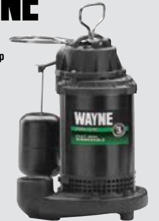
3/4 HP Cast Iron Submersible Sump Pump Heavy-duty submersible pump removes 4,600 GPH at 0' lift. 1-1/2" discharge. Cast iron and stainless steel base. Top suction filters debris. Handle for portability. 406000 $189.99
