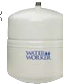
4.4-Gal. Thermal Expansion Tank w/Male Pipe Thread For water heaters up to 80-gal. Controls water pressure build-up and eliminates relief valve spillage caused by thermal expansion when water is heated. 15" H. x 11-1/2" dia. 406139 $69.99
