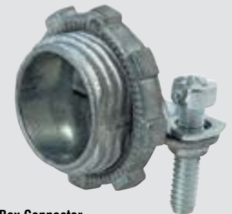
3/8" Box Connector Clamp-type for nonmetallic sheathed cable. Die-cast zinc body. Maximum wire size No. 10-3. For 1/2" KO. UL listed. 509621 79¢
