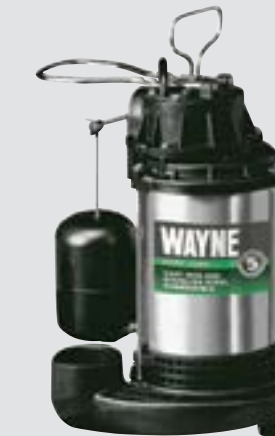
1/2 HP Cast Iron Submersible Sump Pump Float automatically starts/stops pump. Pumps up to 3,720 GPH at 5' lift. 1-1/2" discharge. Operates vertically to save space. Automatic overload. Compact, fits in sump pits as small as 10" in dia. 8' cord. 448370 $179.99
